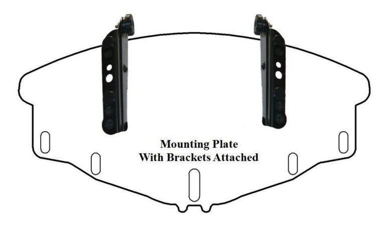
The mounting plate then slides into the fairing in place of the stock shield and screws down with the original factory windshield screws. Leave the factory adjustment levers and strap loose while you do this.
