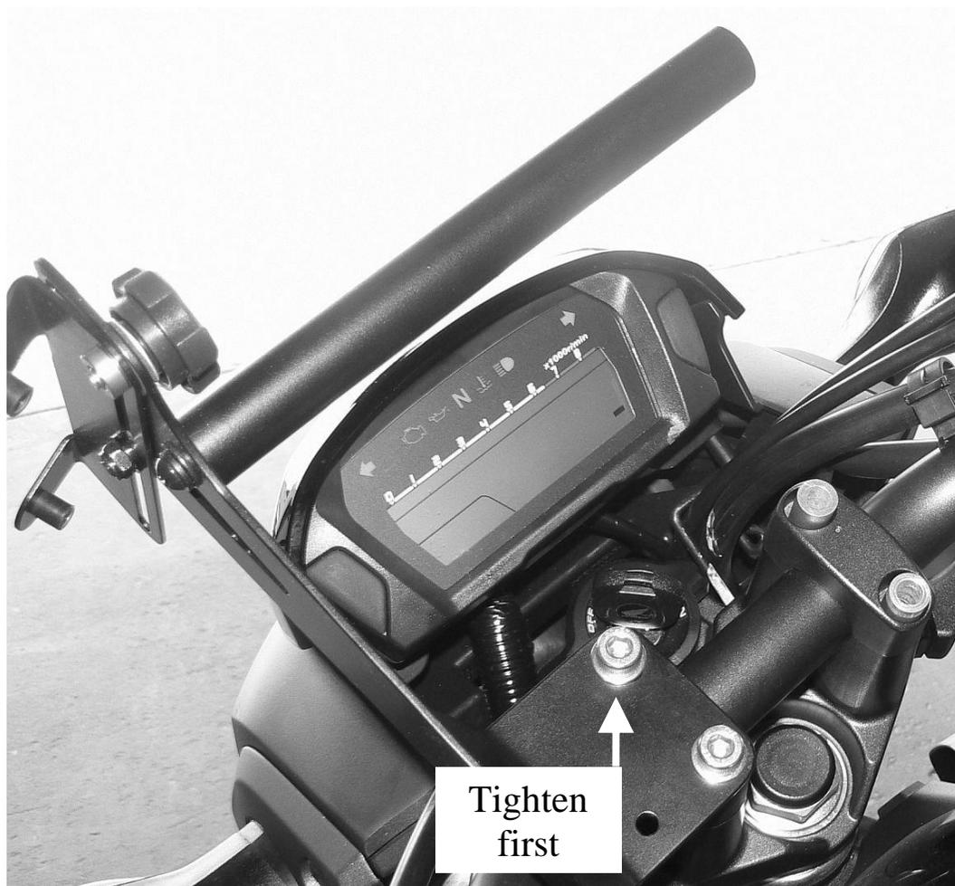
**STEP 6** – Repeat steps 3, 4 and 5 for the other half of the brackets. Don't fully tighten the bar clamp bolts until you fasten the crossbar to the second side. Use the same hardware configuration for this as you did on the other side of the crossbar. Once the crossbar is installed, then finish tightening down the bar clamp bolts same as you did in Step 5.
