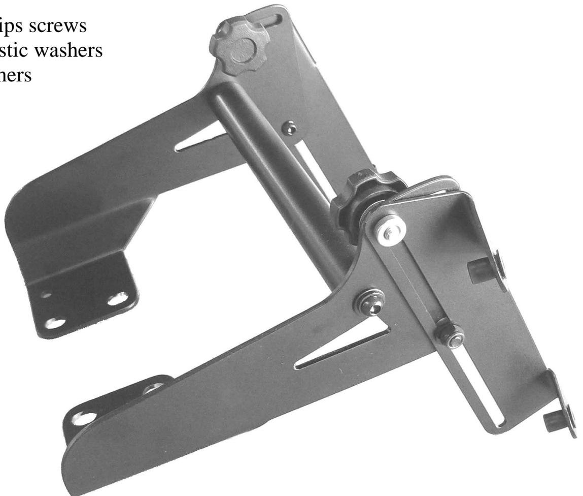
This MadStad system attaches above your handlebar clamps using aluminum spacers and longer bolts. Your handlebars do not need to come loose as you can install these brackets one side at a time.
