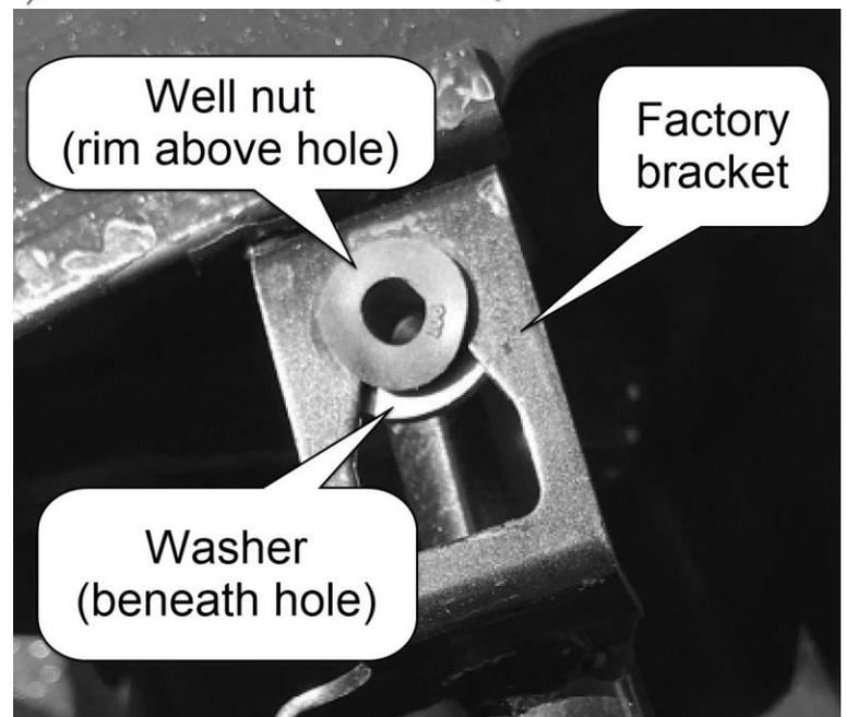
For the upper holes, tilt our well nut assembly into the hole so the washer goes through diagonally. Then slide the well nut upward through the gap to snap it into the round part of the hole.
