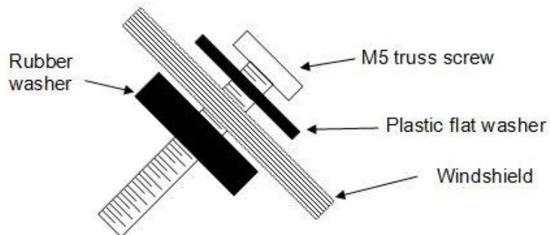
As with the base plate screws, do not overtighten the windshield screws. The rubber well nuts will swell up and when about 1/4 inch of the screw comes out the back side, the windshield should be snug and secure.
