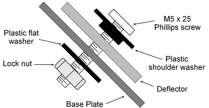
Each side deflector is attached with an M5 screw and shoulder washer (the 2-level washer) in the front and the plastic flat washer and lock nut on the back as shown in the diagram above. Tighten each screw and nut together enough to hold the deflectors on but have room for movement.
