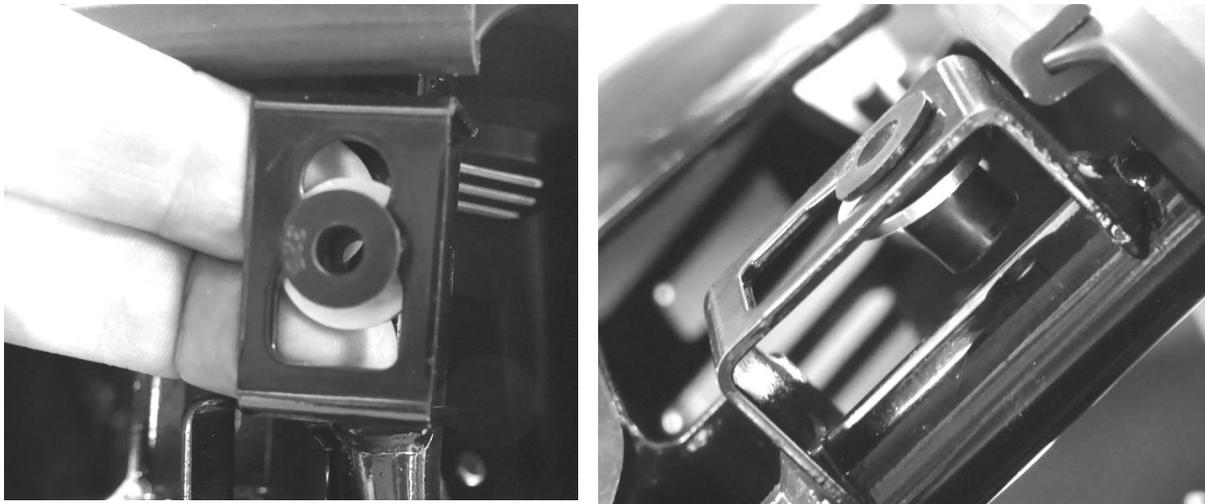
For the lower holes simply push the rubber nuts up through the open gap to snap them in, making sure the rubber rim is on top and the metal washer underneath. *Try and keep the flat washers tight up against the back of the factory hole.*
