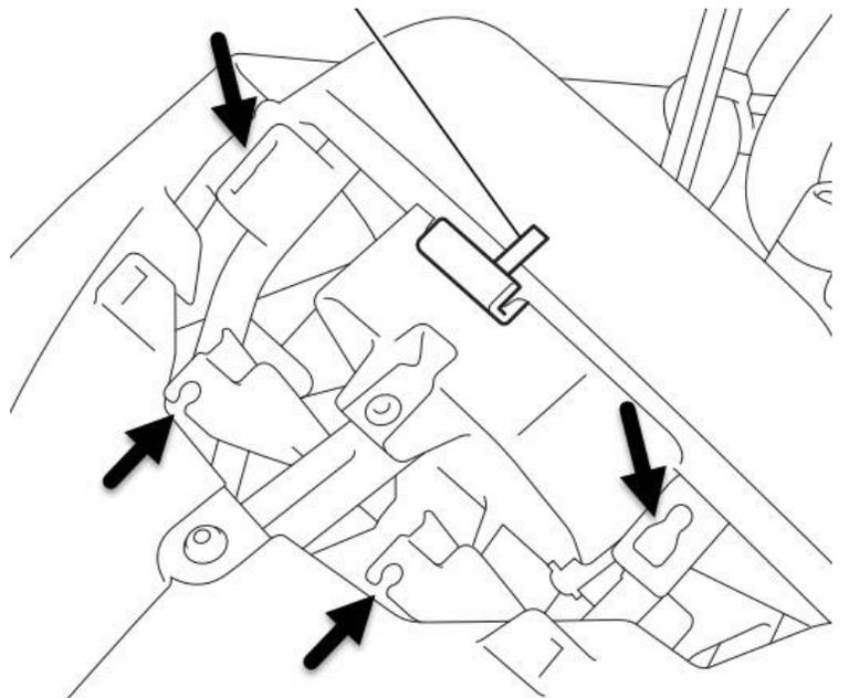
Instead you will insert the pre-assembled rubber well nuts which have metal washers on them. These well nuts slide into the factory slots with the rubber rim of the well nut above the hole, and the metal washer below it as seen at right.
