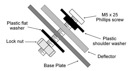
Each side deflector is attached with an M5 screw and shoulder washer (the 2-level washer) in the front and the plastic flat washer and lock nut on the back as shown in the diagram above. Tighten each screw and nut together enough to hold the deflectors on but have room for movement.
