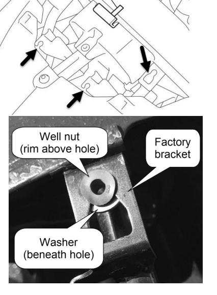
For the upper holes, tilt our well nut assembly into the hole so the washer goes through diagonally. Then slide the well nut upward through the gap to snap it into the round part of the hole.
