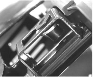
For the lower holes simply push the rubber nuts up through the open gap to snap them in, making sure the rubber rim is on top and the metal washer underneath. Try and keep the flat washers tight up against the back of the factory hole.
