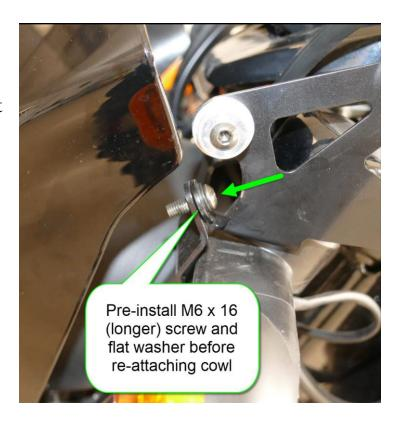
Once both screws are set as shown above, snap the cowl back on at the bottom and use the long-arm hex key wrench provided to fasten the inner screws back
