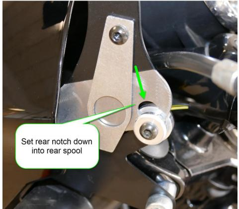
Lift up on the bottom of the locking tab and rotate it onto the rear spool. If it doesn't want to lift, push in a bit on the inside of the spring-loaded screw. Make sure the locking tab is fully seated over the spool. Repeat this on the other side.
