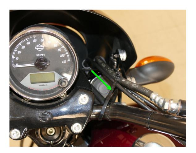
Set the front notch of the adjustable bracket into the front spool of our base brackets as shown here.
