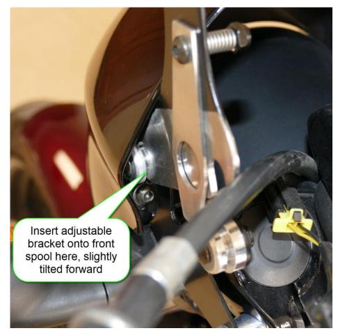
With the front notch slid all the way into the front spool, you will be able to push the rear notch down onto the rear spool. Make sure the pivoting locking tab is out of the way as shown here.
