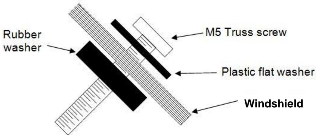
When attaching the shield to the brackets, we recommend that you first install the upper and lower screws on one side, then install the upper and lower screws on the other side. The rubber well nuts are flexible and shield holes are oversized so you can nudge the shield around to align the T-screws with the holes properly. Tighten the screws with a screwdriver until the tips of the screws come out of the bottom of the well nuts, and the well nuts begin to swell up (bulge) behind the brackets.
