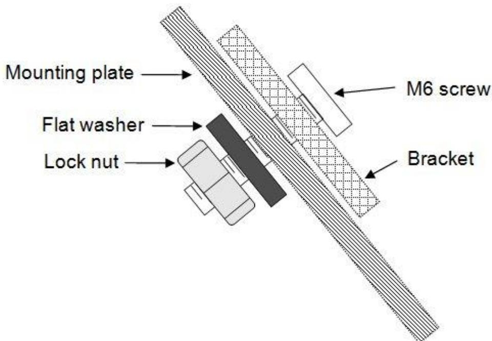
The knobs on the brackets go to the insides (facing each other) with the knob sides up. When both brackets are installed it should look like the diagram below:
