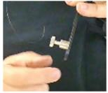
The brackets have two notches on them and those notches slide onto the posts on the support bracket. Slide each one on and make sure both notches are fully seated. You can then release the latch pin by rotating it clockwise until it snaps into the hole on the support bracket. Make sure that the pin is all the way through the fly screen bracket hole because this is what keeps the brackets locked in place. See photos below.
