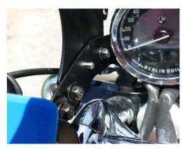
**NOTE:** If the brackets slide onto the posts but seem a bit loose as they go on, tighten the post mounting screws down a little harder. The plastic spool will compress slightly to provide a more snug fit.
