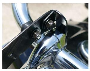
B. Repeat this process with the other handlebar clamp to complete the support brace installation. The finished installation should look like the image at right.
