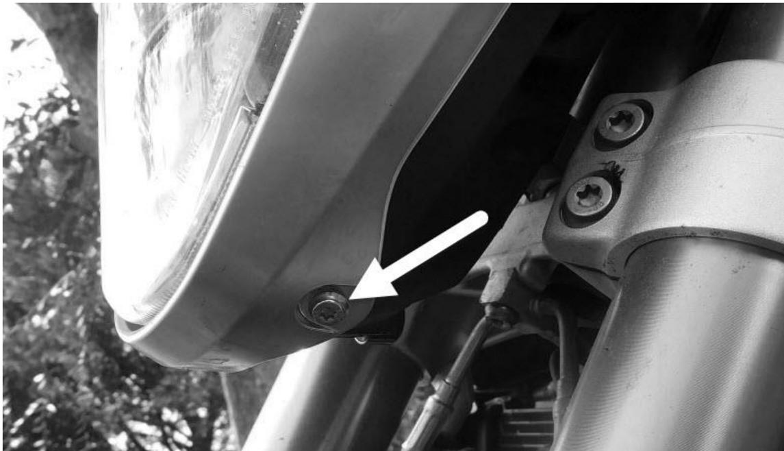
**STEP 2:** Remove the black plastic cover plate which sits beneath the instrument panel (see photo at right).
