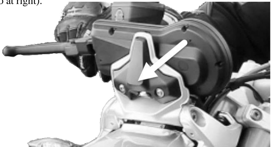
**STEP 3:** Install our base plate as shown below using the short M5 x 12 screws with metal flat washers. See arrows below for screw location. Holes have been provided in the middle of the base plate for screwdriver access to the upper mounting screws.
