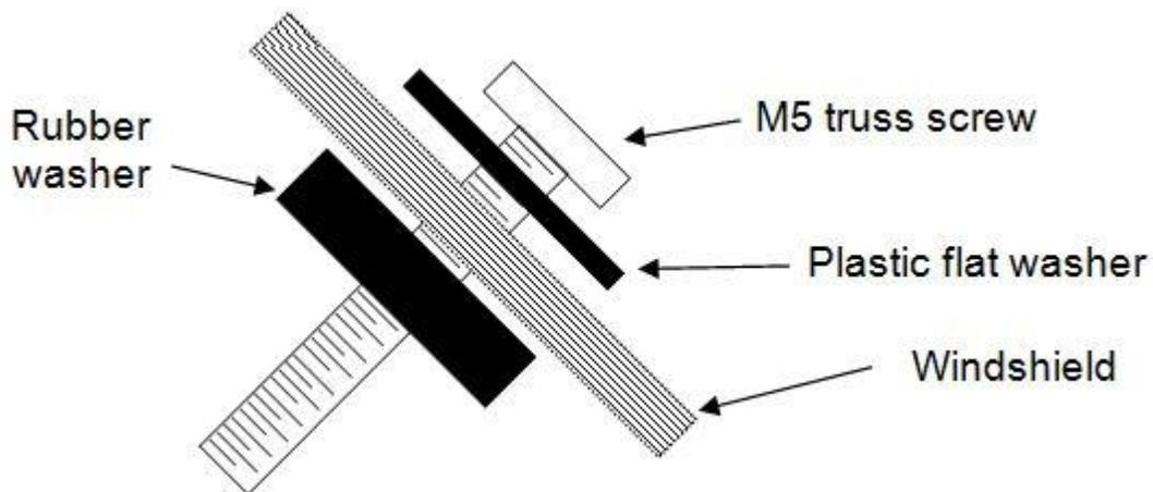
**DO NOT OVERTIGHTEN THE TRUSS SCREWS!** The rubber well nuts cannot be pulled up out of the brackets, even if they are not tight, so tighten only until the well nuts begin to swell up and the shield is snug against the brackets. Over-tightening can damage the rubber well nuts.
