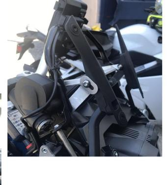
Once the braces are in on both sides and all fasteners are tightened, the factory height-adjust mechanism won't work anymore.
