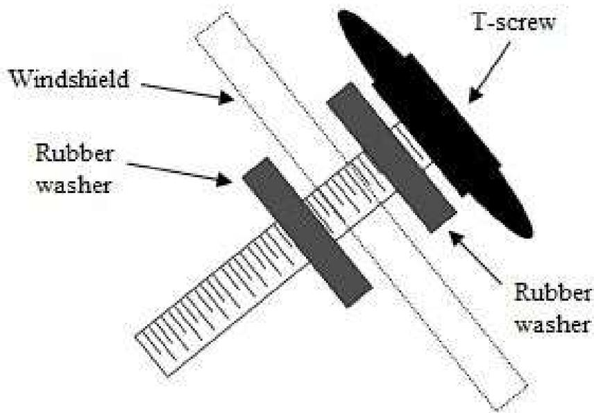
**DO NOT OVERTIGHTEN THE T-SCREWS!** The rubber well nuts cannot be pulled up out of the brackets, even if they are not tight, so tighten only until the well nuts begin to swell up and the shield is snug against the brackets. Over tightening can damage the rubber well nuts.
