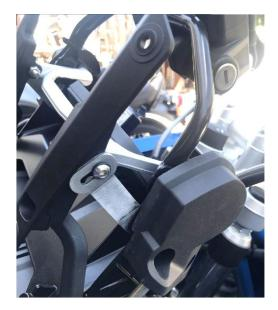
Once the side brace is attached securely to the pivot point at the front, and the side screws and nuts are tightened as well, go ahead and repeat the process on the other side. After that you can put back the flat plastic arms that held the factory shield, you are going to attach our brackets there next.
