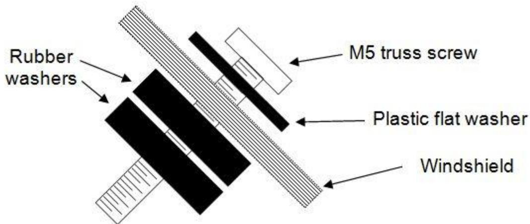
**DO NOT OVERTIGHTEN THE WINDSHIELD SCREWS!** The rubber well nuts are secure in the brackets, so tighten them only until the rubber body begins to swell up and the shield is snug against the brackets. Over tightening can damage the well nuts.
