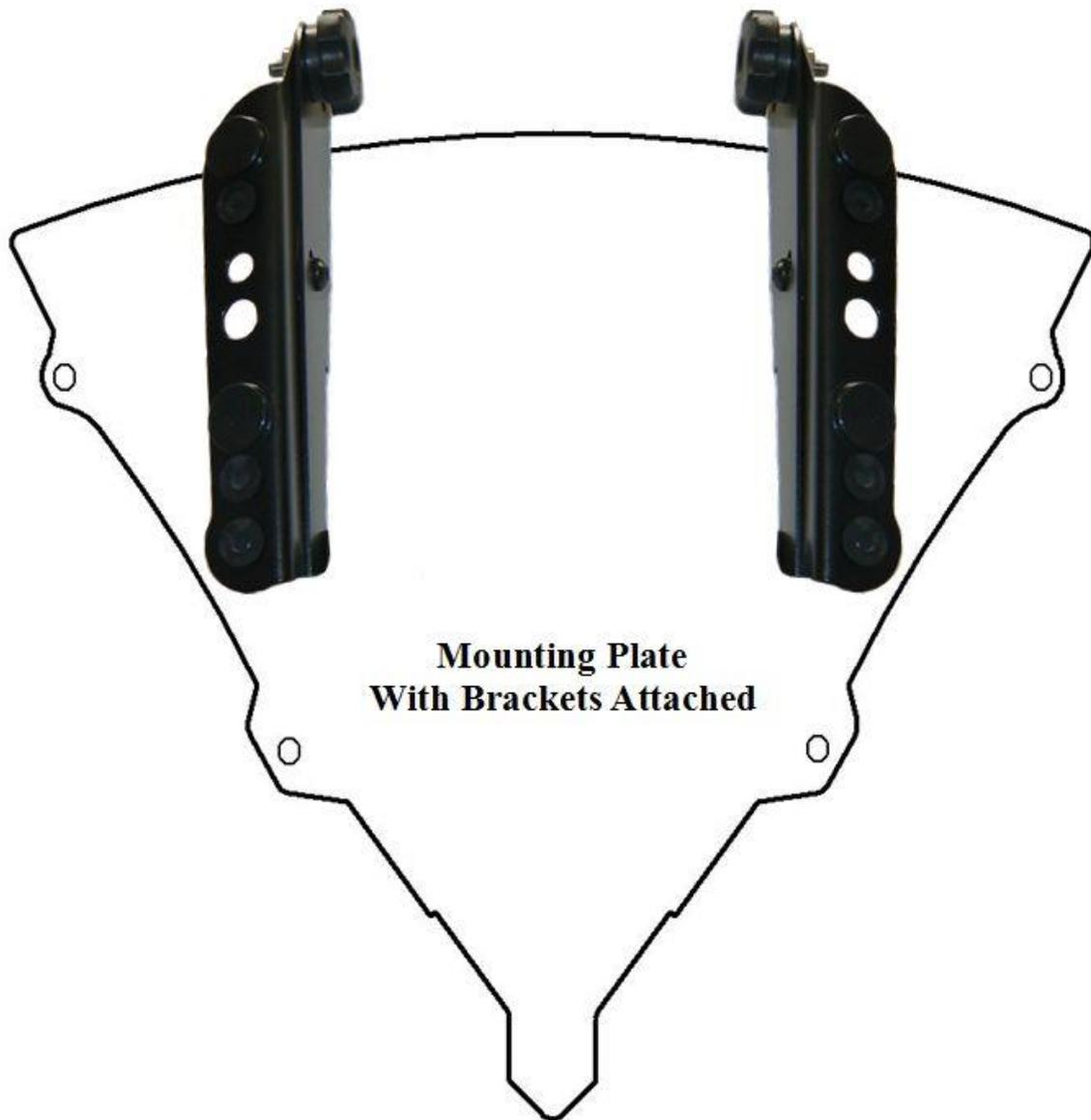
The adapter plate then slides into the fairing in place of the stock shield. Wiggle the nose into the bottom then align the four well nuts with the four holes in the fairing. There will be a slight gap toward the top of each side of the fairing, but this is normal. Screw it in with the original factory windshield screws.
