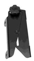
MadStad adjustable brackets are designed to bolt to a curved surface like the metal adapter plate included in this kit. The new windshield attaches to the top of the brackets with quick-removal T-screws. Loosening the two adjustment knobs allow you to change the windshield height and tilt without getting off of the bike, and without any tools.
