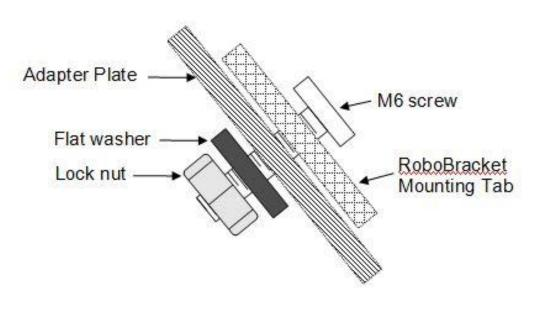
The knobs on the brackets go to the insides (facing each other) with the knob sides up. When both brackets are installed it should look like the diagram below:
