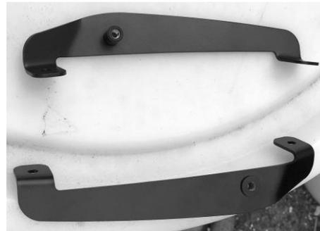
MadStad brackets are designed to bolt to a curved surface like the metal adapter plate included in this kit. The new windshield attaches to the front of the brackets with quick-removal T-screws. Loosening the two adjustment knobs allows you to change the windshield height and tilt without getting off of the bike, and without any tools.
