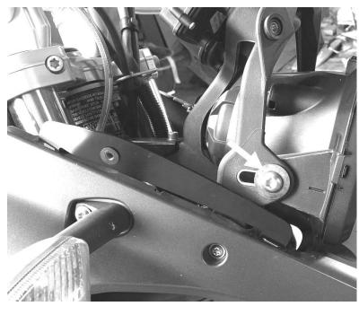
The adapter plate then installs onto the fairing in place of the stock shield using the original factory windshield screws and washers in the front, and the M5 x 25mm Phillips screws with plastic washers that came with this kit. Start with the four front screws and screw them in, but not tightly just yet. Install the two side screws last. You may have to wiggle the adapter plate around or flex it a bit to
