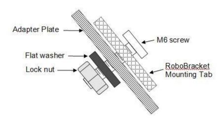
The knobs on the brackets go to the insides (facing each other) with the knob sides up. When both brackets are installed it should look like the diagram below: (your brackets may appear slightly different, this is for orientation purposes)
