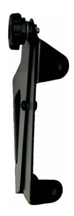
MadStad RoboKnob brackets are designed to bolt to a curved surface like the metal adapter plate included in this kit. The new windshield attaches to the top of the brackets with *M5 Phillips truss screw*, *M5 flat plastic washer*, *windshield then M5 soft rubber washer*. Loosening the two adjustment knobs allow you to change the windshield height and tilt.
