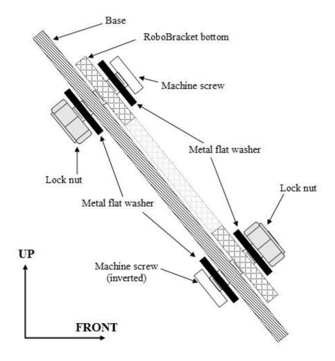
The knobs on the brackets go to the insides (facing each other) with the knob sides up. When both brackets are installed it should look like the diagram at right:
