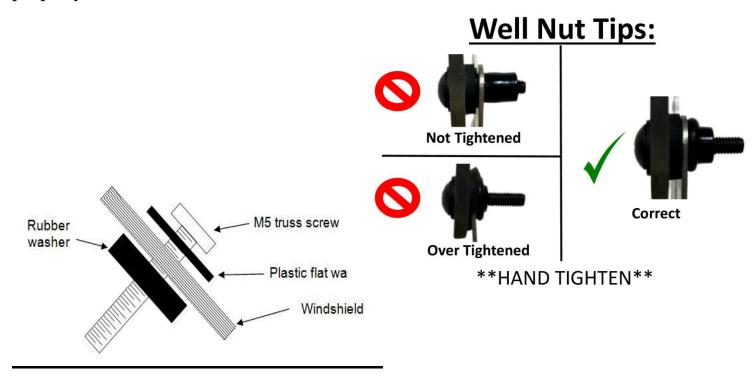
**DO NOT OVERTIGHTEN THE SCREWS!** The rubber well nuts cannot be pulled up out of the brackets, even if they are not tight, so tighten only until the well nuts begin to swell up and the shield is snug against the brackets. Over tightening can damage the rubber well nuts.
