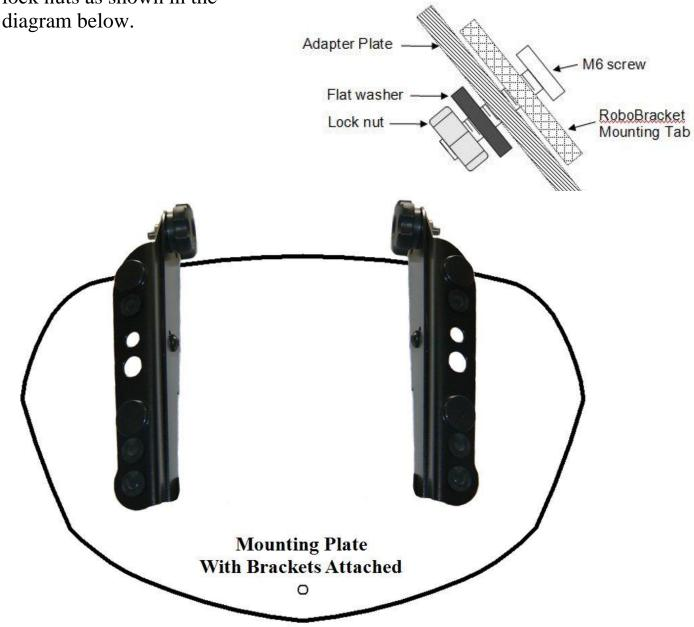
The adapter plate then attaches to the fairing in place of the stock shield, but also attaches on the sides to the turn signal bracket *at the screw above the turn signal*. Remove the factory screws there and use the ones we have provided in this kit. Plastic spacers have been provided which go between the adapter plate and your bike at the top three holes. Here is how to install the adapter plate and hardware:
