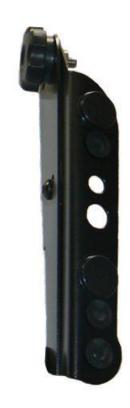
MadStad RoboKnob brackets are designed to bolt to a curved surface like the metal adapter plate included in this kit. The new windshield attaches to the top of the brackets with the provided truss M5 screws. Loosening the two adjustment knobs allow you to change the windshield height and tilt without getting off of the bike, and without any tools.
