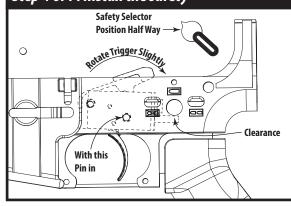
4a) With only the rear pin in the trigger, rotate the trigger assembly as shown, so the safety will not interfere when being inserted.
