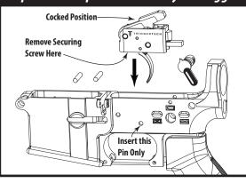
**CAUTION:** Be careful when removing the plastic securing screw as the trigger can rapidly release. Support the hammer and housing at all times.
