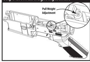
**IMPORTANT**: Some TriggerTech models allow you to adjust your trigger pull weight. The set screw located towards the rear-center of the trigger can be adjusted using the supplied 3/32" Allen wrench. Factory setting is approximately 3.5 lb. We recommend getting used to the factory setting before adjusting the pull weight down. Always keep the set screw engaged with two to three "clicks" otherwise it may fall out during use.
