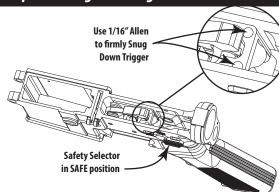
**IMPORTANT:** It is **CRITICAL** that you firmly, and **PROPERLY**, tighten **BOTH** Snug Down screws prior to re-assembling your firearm.
