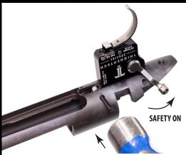
4a) Insert the trigger assembly and gently tap the front trigger pin in, from right to left. Ensure that the pin is not contacting the bolt release as this can jam the bolt catch, which is dangerous.
