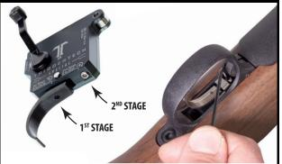
Your TriggerTech trigger is set near the middle of the advertised pull weight range and can be adjusted in increments. To adjust pull weight, insert the supplied 5/64" Allen wrench into the set screw located at the bottom of your trigger. To increase pull weight, rotate the set screw clockwise. Pull weight varies between actions.
