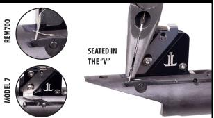
5a) If you have a bolt catch, adjust the bolt release to the bolt catch by using a pair of narrow pliers and gently bend the tab until it slots perfectly into the bolt catch notch. At rest, the bolt release should be seated in the "V", as shown. This may take several attempts.
