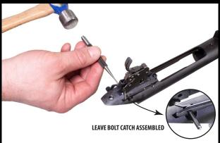
2a) Gently tap the front trigger pin from left to right until the trigger assembly becomes free.
