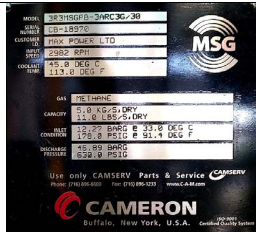
GBC Compressor Nameplate
