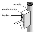
Unscrew the handle mounts through the holes on the inside of the door frame, and remove the handle.
