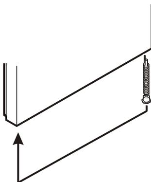
15. Suspend the freezer door on the hinge pin and close.
