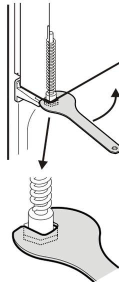
10. Reinstall the middle hinge bracket on the left-hand side.
