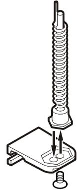
4. Unscrew the pin on the middle hinge bracket.
