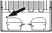
**Sensor cable opening for freezer compartment**
