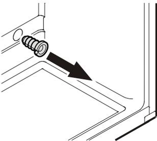
Pull out strain relief device.
