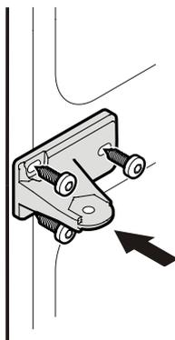
14. Screw the hinge pin into the middle hinge bracket.
