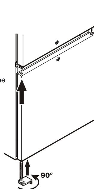
16. Install the lower hinge bracket.
