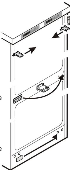
13. Turn the refrigerator door spring mechanism anticlockwise using the open-ended spanner provided, until the hexagon engages in the recess of the middle hinge bracket.
