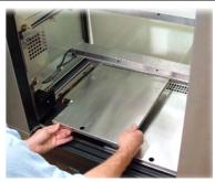
7. Both door guide bottom runners can be lifted out for cleaning.
