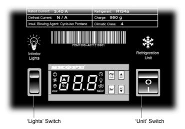
Cabinet All three interior lights will operate continuously unless they are manually **Lighting** switched off using the 'Lights' switch on the left hand side of the controller. The cabinet fluorescent lights will require a period of time to stabilise following initial start up.
