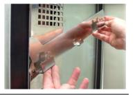
Refit the shelf support panels, light panels and wire shelves. Refit the sliding doors by lifting each door up into the top track and placing onto the bottom track.
