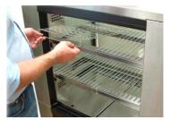
Remove the shelf rear support panels and shelf lighting panels by lifting up off the shelf brackets. The lighting panels have power cables connected to the cabinet, limiting how far they can be pulled out from the cabinet.
