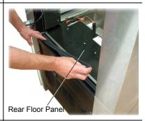
8. The evaporator drain should be regularly checked and cleaned to prevent blockage. To access the drain hole, remove the rear floor panel from inside the cabinet (see photo above). If using water to clear the drain, care should be taken not to overflow the condensate tray (see below).
