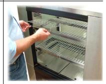
4. The shelf rear support panels and shelf lighting can be removed from the cabinet by lifting up, off the shelf brackets. The power supply cable will remain attached to the lighting panels.
