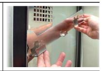
6. The floor panels can be removed from the cabinet by lifting each panel up.
