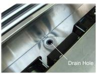
9. The evaporator drain tube should also be checked for blockage. To access the drain tube, remove the ventilation panel from the rear of the cabinet by undoing the two bottom screws and unhooking from the cabinet. To clear the drain tube, pull the drain tube out from the cabinet and drain the water into a bucket.
