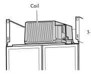
Brush the condenser coil with a soft brush to remove any dust and fluff.
