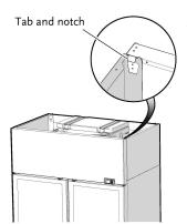
Refit the sign assembly and reconnect to the power supply.
