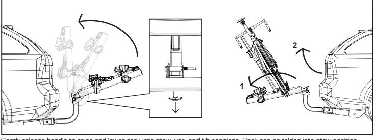
Gently release handle to raise and lower rack into stow, use, and tilt positions. Rack can be folded into stow position when now in use and tilted down for rear vehicle access. Load arms should be stowed flat when rack is not in use. Handle should be fully seated before each use.
