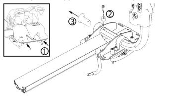
Flip load arm and reinstall from the other direction.
