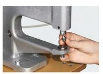
Replace the upper and lower die in order to apply the Snap Fastener closure.
