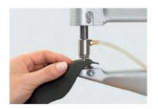
Position the carrier material and apply. Regulate the offset/pressure using the adjustable stop.
