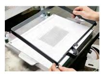
12 Place the black frame on the masks. The frame makes sure no Back Parts get lost.
