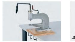
The **fly press** (art. 9040/019, with mounting board) represents an easy way to mechanically apply the products.
