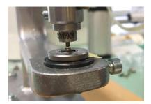
Before starting the application make sure that upper and lower die are positioned in the center. Pre-punching the fabric and positioning it properly on top of the lower die guarantees the correct functionality of the finished product.
