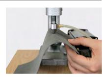
Position the carrier material with the right side pointing downwards. Apply the 3D Stud by carefully closing the handle of the fly press.
