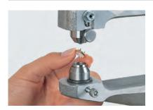
Place the Decorative Button/upper part of the Snap Fastener in the lower die, with the claws pointing upwards.
