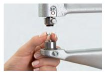
Place the pronged ring in the lower die, with the prongs pointing upwards.
