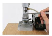
2 Attach the vacuum pump to the upper die and turn the vacuum pump on. The Back Part can now easily be positioned into the upper die with the arrow pointing downwards.
