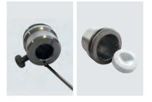
2 Use the changing pin to slowly slide the plastic insert out of the attaching die from above, through the small hole at the edge.
