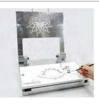
2 Sieve Rose Pins into the mask with the claws pointing upwards. Use one mask for each Rose Pin size and repeat the sieving step with all masks.
