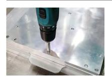
Before starting production with a new motif, the vacuum suction has to be installed in the mold. Open the cover's plates by unscrewing the screws with a drill.
