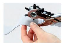
Pre-punch the carrier material on the designated position for the Crystal Stud.
