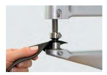
3 Apply the product to the textile in the previously marked position, ensuring it is on the right side of the fabric. Regulate the offset/pressure using the adjustable stop.
