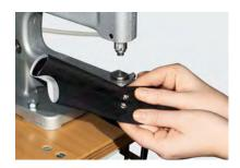
Apply the product on the carrier material. Adjust the offset/pressure using the adjustable stop. Check the functionality of the Snap Fastener after the application.
