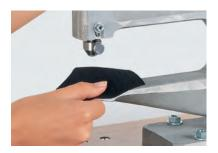
3 Apply the product to the textile in the previously marked position. Regulate the offset/pressure using the adjustable stop.
