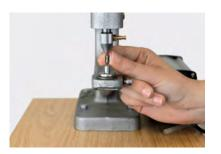
Place the 3D Stud in the lower die, with the crystal side pointing downwards.
