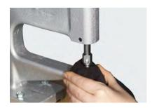
Apply the product on the carrier material. Adjust the offset/pressure using the adjustable stop.
