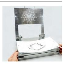
After having sieved all Rose Pins into the mold, remove the masks.
