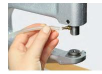
**3** Connect the vacuum pump and turn it on.
