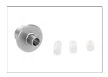
3 Choose the matching insert for applying a 3D Stud of another size and push it into the lower die. Make sure the cavity of the insert is located at the upper side of the tool.
