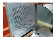
4 The mold is now ready to be equipped with the PVC masks. First open the mold.
