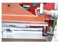
17 Close the cover and place the mold into the hydraulic press.
