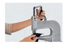
Carry out the application in the desired position. Regulate the offset/pressure using the adjustable stop.
