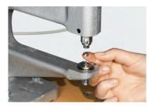
Place the ball part in the upper die (will be kept in position by vacuum) and the counterpart in the lower die.
