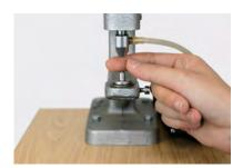
Set a 3D Stud (crystal pointing downwards) in the lower die with insert.
