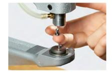
Place the upper part in the upper die (crystal pointing upwards).
