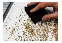
13 Empty the Back Parts into the black frame. Use the sponge to wipe them into the mask's cavities (arrows pointing downwards).
