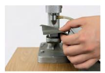
3 Turn the fabric with linear grid around and put all parts into the fly press on top of the lower die. Activate the vacuum pump and fit the Back Part into the upper die. Apply the 3D Stud by closing the handle of the fly press.
