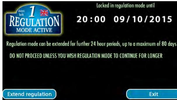
Press **Extend regulation** and you will be given the option to enter the number of days that Regulation Mode should be extended for. The default, zero, will NOT enter regulation mode, even if **Confirm** is pressed.
