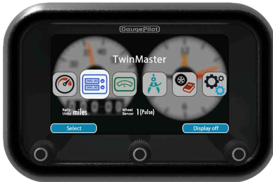
Your GaugePilot instrument is controlled via its three front knobs. These can be rotated left and right, and pushed.
