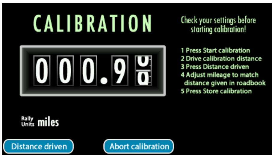
At the end of the calibration distance, press [Distance driven](#).
