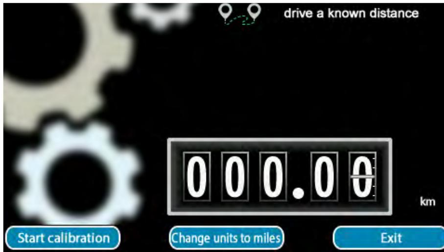
At the start of the calibration distance, press **Start Calibration**. If a previous calibration had been started and completed or aborted, the odometer will automatically reset itself to 0.
