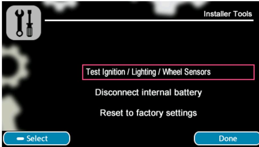
The highlighted option is selected with a long press of **Select**. Turning any knob scrolls the highlight window. Selecting **Done** exits the installer tools.
