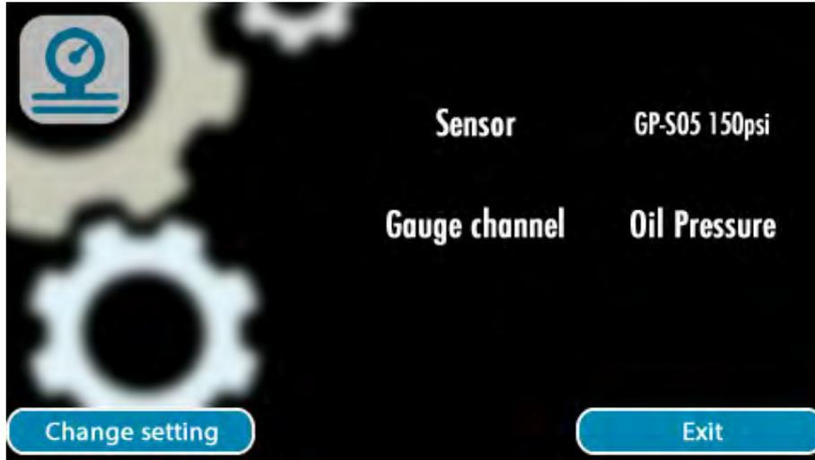
The pressure input allows connection of a 3-wire 5V powered sensor, providing a 0-5V input signal, for measuring Oil Pressure, Fuel Pressure, or Boost.
