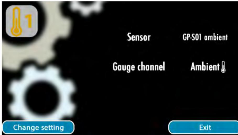
Temperature input 1 allows connection of dedicated 2-wire resistive sensors for measuring Ambient, Coolant, Oil, or Intake temperature.
