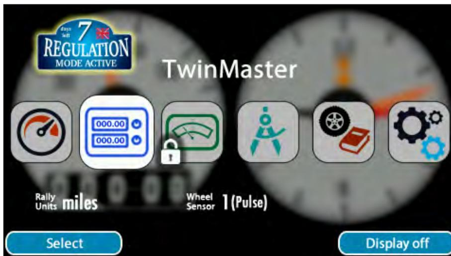
Once a GaugePilot is in Regulation Mode there is no way to remove it from Regulation Mode other than waiting for the time-based lock to expire. Changing the time or date, removing the internal backup battery, performing a factory settings reset or firmware update, or switching Car ID will not remove, or accelerate removal, of Regulation Mode.
