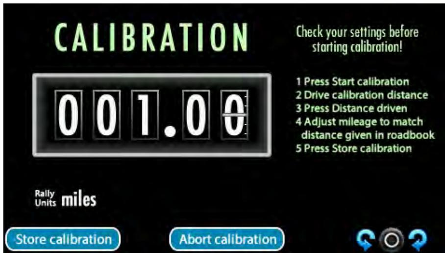
Press **Store Calibration**, which doesn't appear until a knob is turned. If the displayed mileage is already correct, turn the knob left a click and then right a click so that the instrument can see that you've corrected the mileage and it will then offer you the ability to **Store Calibration**.
