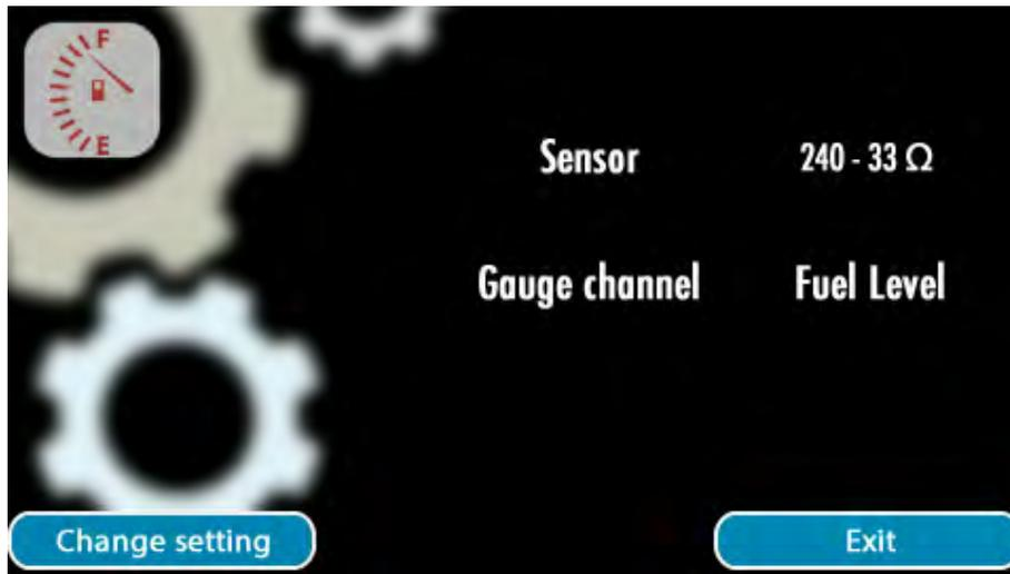
The fuel sender input allows connection of a 2-wire resistive sensor to measure fuel level. This sender must NOT be connected to any other device in addition to GaugePilot - this feature is targeted at vehicles currently without a fuel gauge and for which the addition of a fuel sender is desirable.
