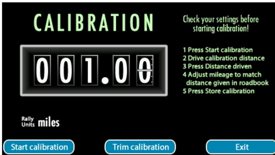
Once stored the calibration is used until another calibration is performed. If happy with the calibration select **Exit** or otherwise perform another calibration using **Start Calibration** having driven back to the start of the distance.
