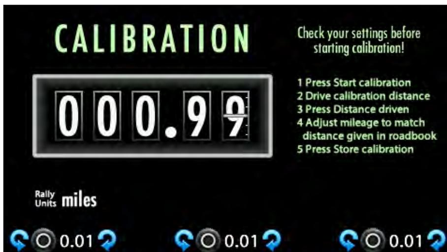
Turn any knob to change the displayed mileage to the correct mileage according to the rally organiser's roadbook. Each turn of a knob will adjust the distance by 0.01 of a unit.
