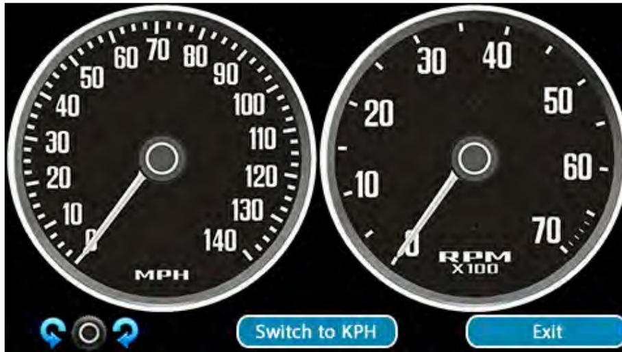
On starting the **Gauges** application, the first gauge pair will be displayed. If more than one gauge pair is defined, rotating any knob will move to the next pair (clock-wise) or the previous pair (anti-clockwise).
