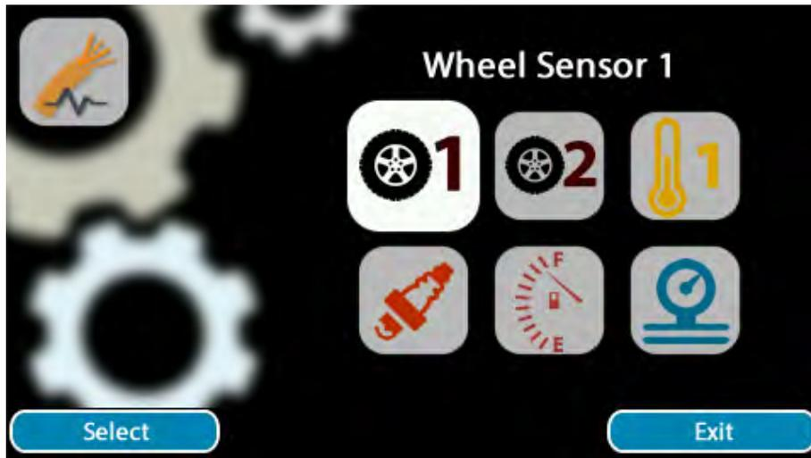
Setup of all directly connected sensors is performed here, including initial settings for the wheel speed sensor(s).
