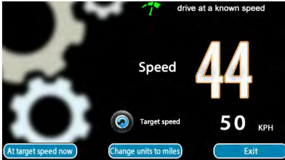
If you don't have a local measured mile that you can use to calibrate your wheel sensor, you can calibrate it by driving at a fixed speed against a known accurate speed reference such as a portable satnav. The target speed can be in mph or kph - If you wish to change the units being used select [change units to miles](#) or [change units to km](#).
