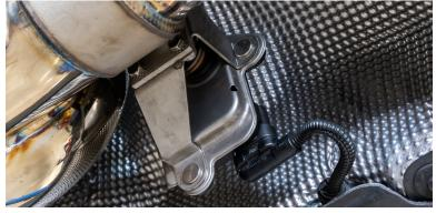
Make sure to disconnect the valve module from the OE exhaust and re-install them on the RE-MARK valve bracket before installing the exhaust on the car.
