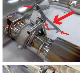
assembly should closely line up with the three bracket holes. Secure valve motor assembly to exhaust valve bracket with the original M8 hardware. Torque to factory spec or ~20 ft-lbs
