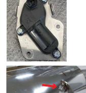
The exhaust valve in the REMARK exhaust is spring loaded and is closed at rest. To properly install the OEM exhaust valve motor, we need to ensure the valve and motor are properly aligned. To do this, we need to manually open the exhaust valve by rotating the actuator plate clockwise until the exhaust valve
