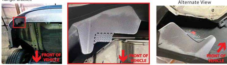
6. Install the REMARK exhaust hanger bracket [6] on the driver's side of the car. This requires removal of the two M8 bolts holding the bumper support beam. Install the bracket and use the provided M8 hardware [5]. Torque to ~20 ft-lbs
