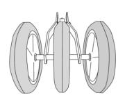
Our heavy duty swivel extension bolts to rear of triple system allowing wheels to track more accurately through turns
