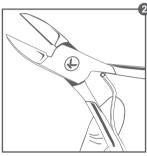
Lift up the spring so it will push against the lever on the opposite side. This spring will help to open up the clipper and your hand
