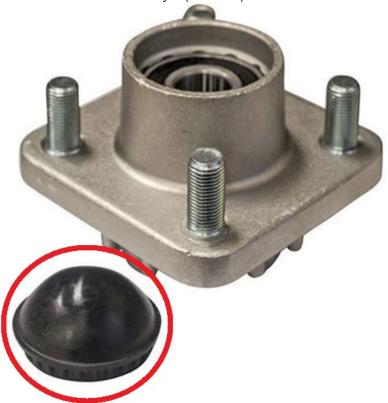
If you cannot determine whether your dust cover is plastic or metal (due to excess grease or dirt buildup), you can simply tap the dust cover with a screwdriver and you should be able to tell what material it is made out of based on the sound it makes (metal covers will "ting" or "ping"). Or, if you have a magnet handy, hold it up to your dust cover to see if the magnet reacts (indicating metal) or not (indicating plastic).
