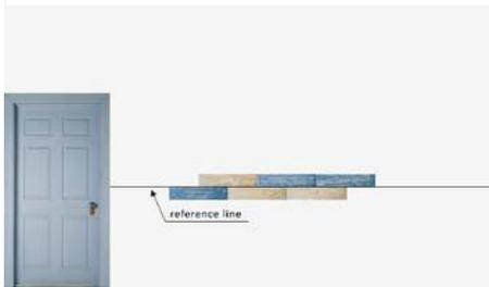
Add more panels above and below the reference line as pictured above. Make sure that the ends of the panels are in good alignment and that there are not large gaps between them.
