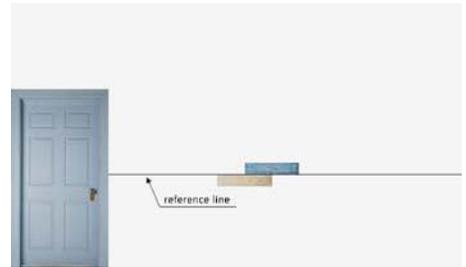
Install one panel above the reference line. Install the other panel below the reference line at the halfway point of the first panel. Once each piece is installed to the wall, it is very important to ensure proper adhesion between the adhesive tape and the wall.
