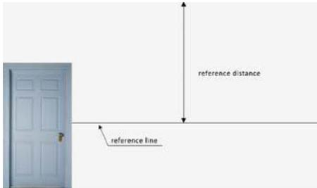
Using a light pencil or chalk, draw a straight line on your wall to help position the first mywoodwall™ panels.
