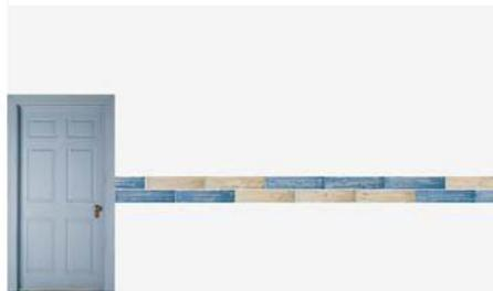
Continue adding panels above and below the reference line until the length of the wall is covered with panels.
