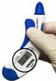
Figure 3 - Tono-Pen AVIA Verification Pass
