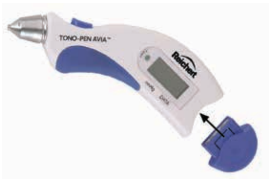
Figure 4 - Tono-Pen AVIA POWERCEL Battery Installation and Replacement
