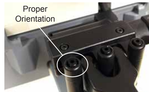
Figure MM-11 Replaced Pen
