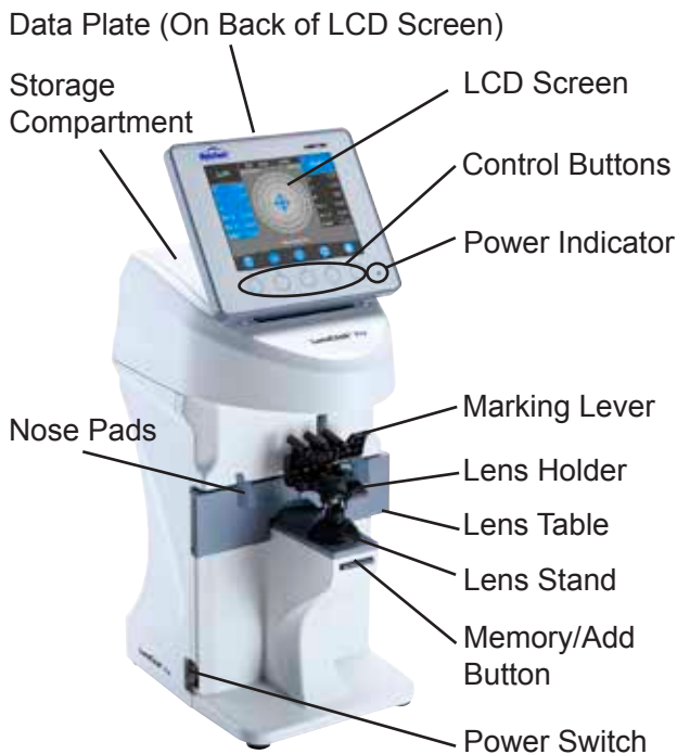
Figure SU-05 LensChek Plus/Pro Front and Sides
