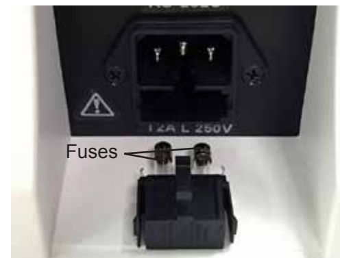
Figure MM-05 Replace Fuses
