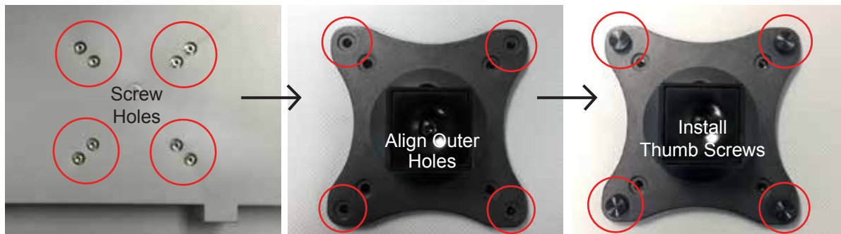
Figure SU-10 Align Holes and Attach Mount
