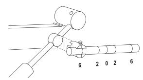
Fig. 18: Check weight - e.g. at measuring drum setting 6
