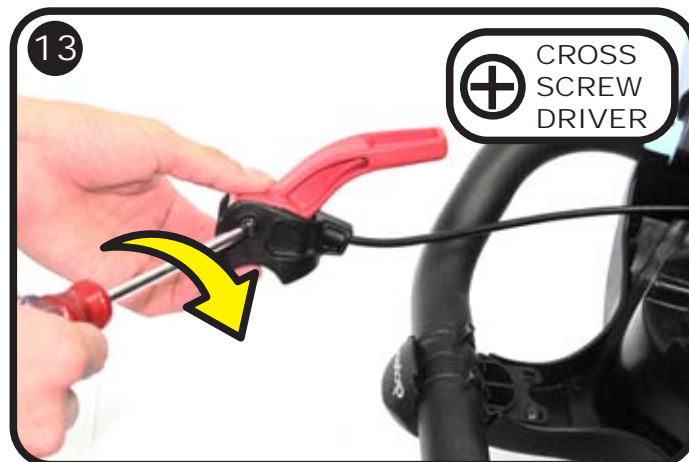
Assemble the Brake Lever on New Umbrella Brake Mount, push the end of the New Brake Cable Sheath and Brake Washer into it.
