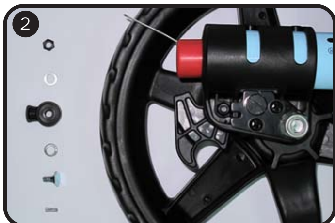
Disassemble the Cable Nut Assembly and remove all the components from the Cable.
