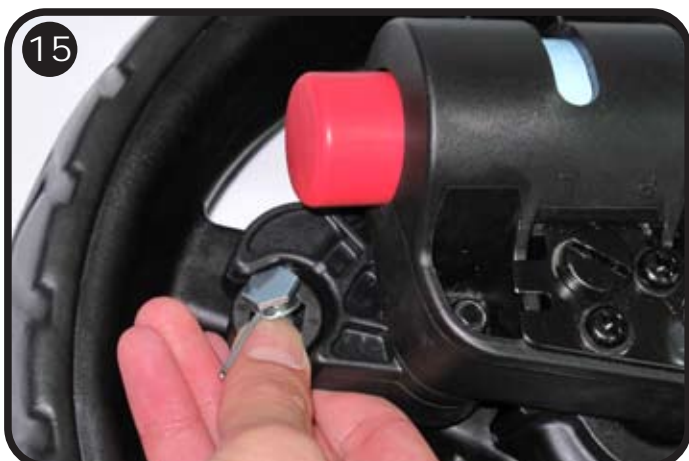
Push the cable bolt with one (1) washer into the brake hammer with the washer between the cable and plastic. Then install the second washer and lock nut on the opposite side of the brake hammer.
