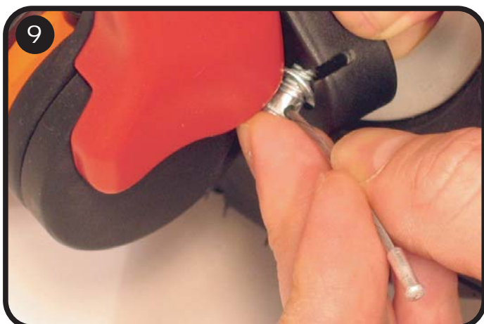
9 Push the cable bolt with one (1) washer into the brake hammer with the washer between the cable and plastic. Then install the second washer and lock nut on the opposite side of the brake hammer.
