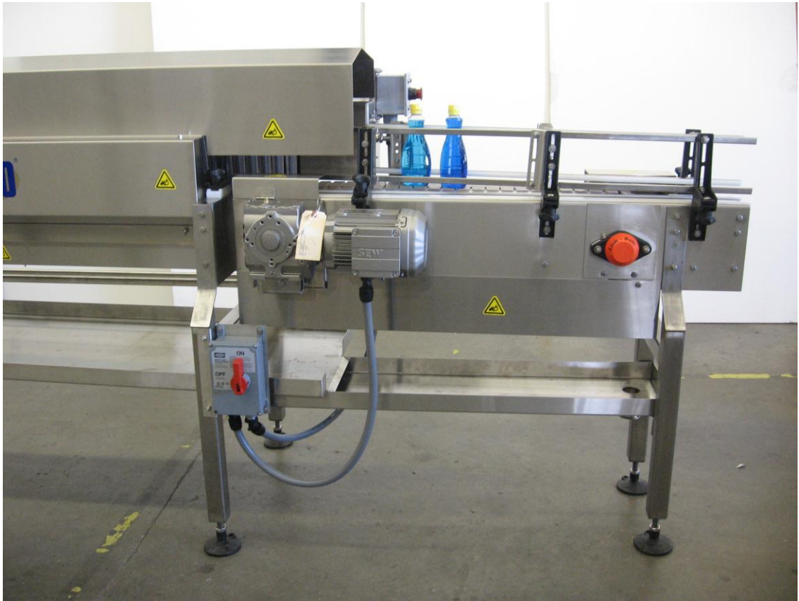
INFEEED END TRANSFER, MOTOR AND DISCONNECT
