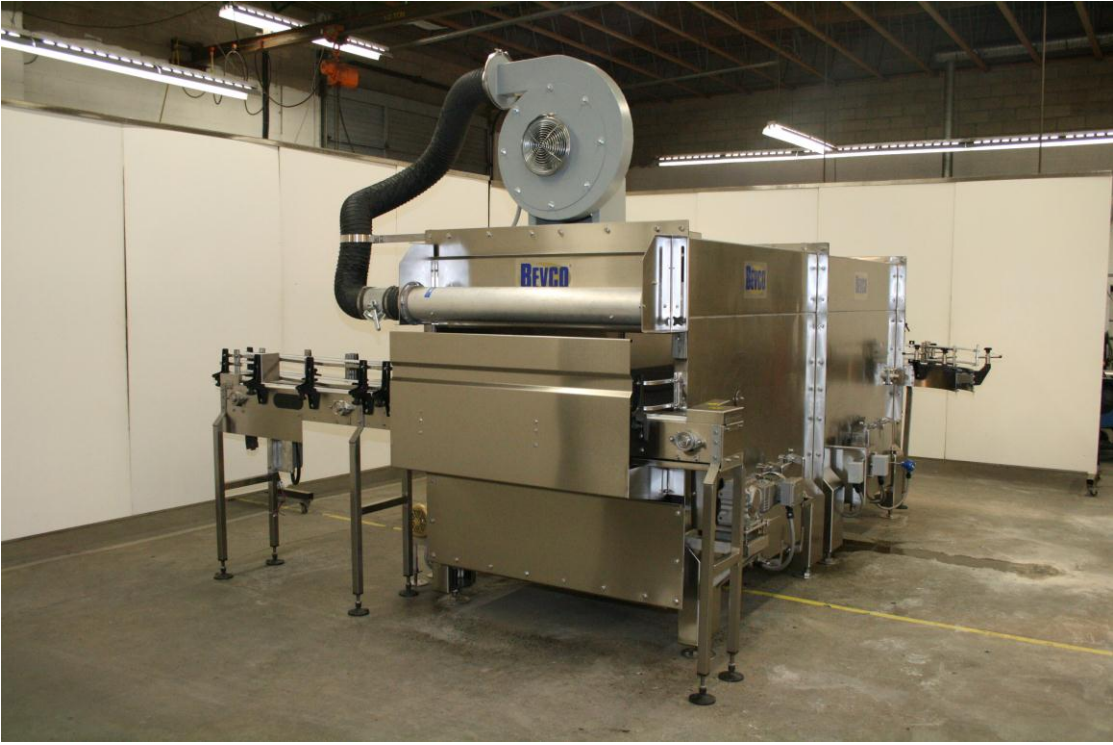
OVERALL VIEW OF COOLER
