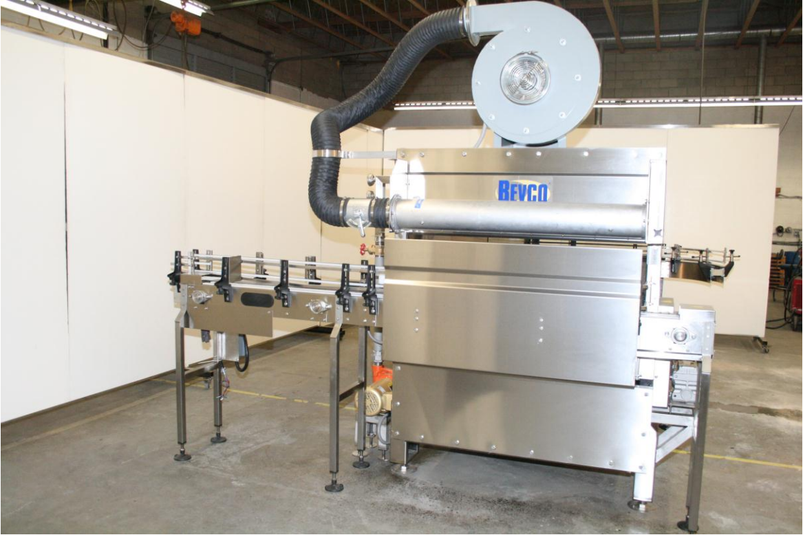
OUTFEED END OF COOLER
