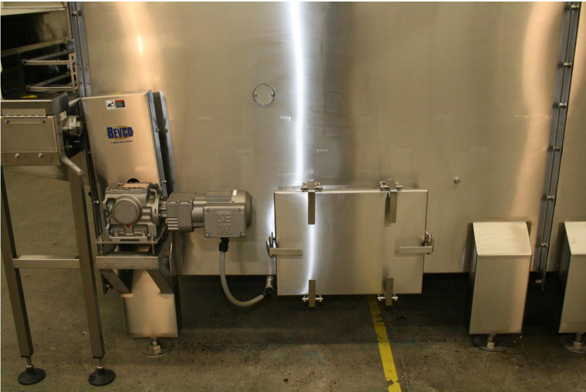
CLEAN OUT DOOR ON DRIVE END
