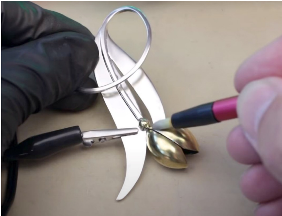
Adding gold highlights to a sterling silver flower. Effects like this are easy to achieve with the pen. Note the attachment of the crocodile clip.
