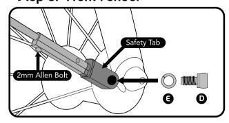
With a 4mm Allen wrench, attach the safety tabs to the eyelets on both sides of the fork with 10mm bolts (D) and lock washers (E). Hold the safety tabs as you tighten the bolts to prevent rotation. Tighten until snug. Do not overtighten. With a 2mm Allen wrench, loosen the 2mm bolts on the safety tabs and position the fender a safe distance from the tire (at least 6mm). Tighten the 2mm bolts on the safety tabs and the two 3mm bolts that connect the stays to the fender.
