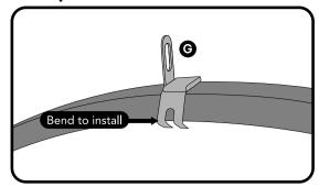
Slide the rear bracket (G) onto the rear fender. Using a pliers, crimp the four tabs on the bottom of the rear bracket (G) to the underside of the rear fender. Crimp tabs until rear bracket is snug, but still able to be moved back and forth on the rear fender for positioning.
