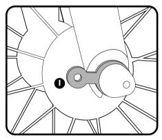
If your bike has threaded eyelets to bolt fender stays to, skip to Step 3. If your bike does not have threaded eyelets, remove the wheel skewer and install an eyelet (I) on each side of the wheel. Reinstall the wheel with eyelets (I) facing the rear of the bike. Make sure wheel is all the way in before tightening skewer.
