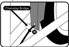
If your bike has a chainstay bridge, use one zip tie (H) to affix rear fender to the chainstay bridge. If you are really lucky your chainstay bridge may have a hole to bolt the fender directly to.
