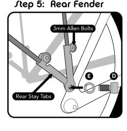
With a 4mm Allen wrench, attach the rear stay tabs to the eyelets on both sides of the dropouts with 10mm bolts (D) and lock washers (E). With a 3mm Allen wrench, loosen the 3mm bolts on the safety tabs and position the fender a safe distance from the tire (at least 6mm). Tighten the 3mm bolts on the safety tabs and the four 3mm bolts that connect the stays to the fender.
