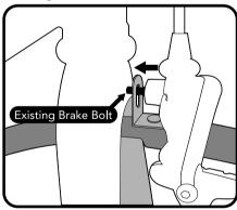
If your bike has caliper brakes, remove the front brake and reinstall with the front bracket between the brake and the fork crown.
