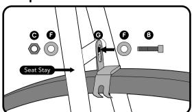
If your bike does not have caliper brakes, use the 25mm bolt (B), two large washers (F) and a Nyloc nut to bolt the rear bracket (G) to the seatstay bridge in the order illustrated above.
