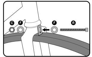
If your bike does not have caliper brakes, use 45mm bolt (A), two large washers (F), and a Nyloc nut (C) to bolt front fender to the fork crown in the order illustrated above. If you don't have a hole in your fork crown, run two zip ties (H) through the front bracket and over each side of the fork crown.
