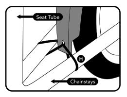
If your bike has no chainstay bridge, use two zip ties (H) to either affix the fender to the chain stays or to the seat tube.
