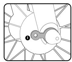
If your bike has threaded eyelets to bolt fender stays to, skip to Step 5. If your bike does not have threaded eyelets, remove the wheel skewer and install an eyelet (I) on each side of the wheel. Reinstall the wheel with eyelets (I) facing the rear of the bike. Make sure wheel is all the way in before tightening skewer.
