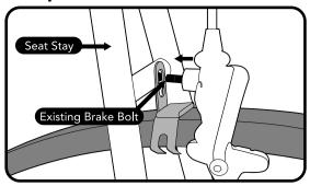
If your bike has caliper brakes, remove the rear brake and reinstall with the rear bracket (G) between the brake and the brake bridge.
