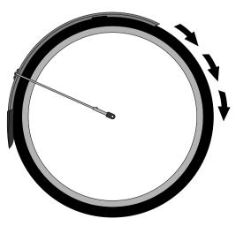
Spin the wheel and check for rubbing and adjust as needed. Double check that all hardware is tight.
