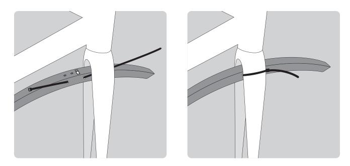
Unfortunately, this will not work for the 30mm or 37mm road fenders because the fender ends up hanging too low and rubbing.
