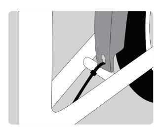
• If you don't have a chainstay bridge at all you can run two zip ties through the hole in the fender and around each chainstay. Make sure to tighten the zip ties evenly so the fender is centered on the tire.
