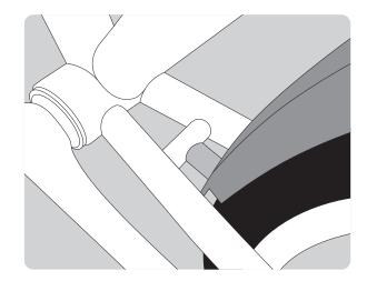
• If you have a chainstay bridge with no threaded eyelet you should still be able to run one burly zip tie through the fender and around the bridge without any trouble.
